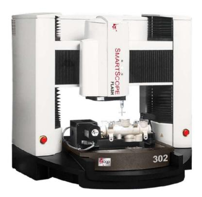
Multisensor Dimensional Measuring System that fits on a Benchtop
