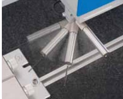
Swiveling of the roughness probe for transverse measurements
