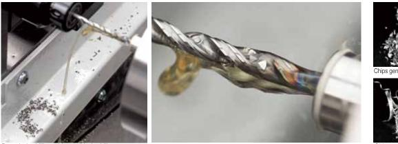
Deep hole drilling with an oil hole drill Since the broken-up chips are expelled along the grooves in the drill, there is no concern about entanglement of chips.
