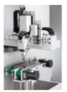
Pallet Conveyor This is a conveyor suited to the feed/conveyance of irregularly shaped products, and precision parts that must not be scratched.
